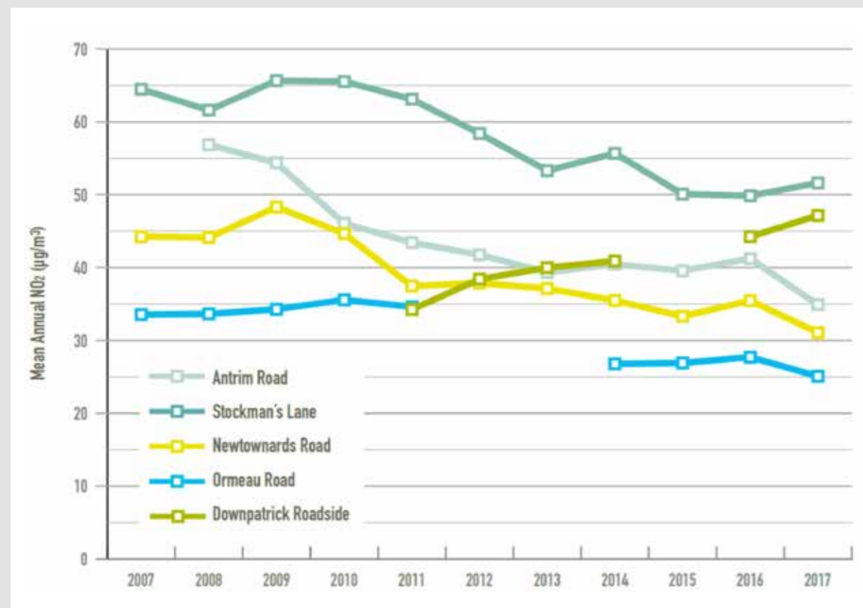
Figure 21. Mean annual NO2 values for five roadside automatic monitoring stations in Northern Ireland, 2007-17
